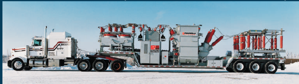
Mobile substation 20 MVA, 115-67 kV/13.2-26.4 kV 95°C winding rise
